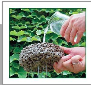
Figure 1: Image of water seepage through porous concrete.<sup>53</sup>
