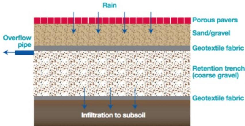
Schematic of porous asphalt and the infiltration of stormwater into subsoil.<sup>67</sup>
